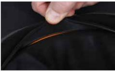
**1.7** Check that the Lock Ring is in position by following the groove 360°.
